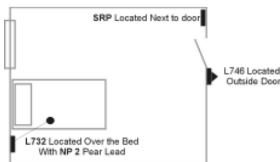
Above: Typical Room Layout showing L732 Call Point, SRP Remote/Preset Unit and L746 Overdoor Light.
